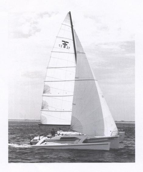
commonly used in multihulls, it being broader and flatter with little rocker and a maximized waterline. This encourages early planing and high reserve buoyancy in the ends discourage any pitching. A major benefit of this shape is a tendency to send any spray horizontally outwards, and this combined with molded-in spray deflectors gives a very dry ride.
