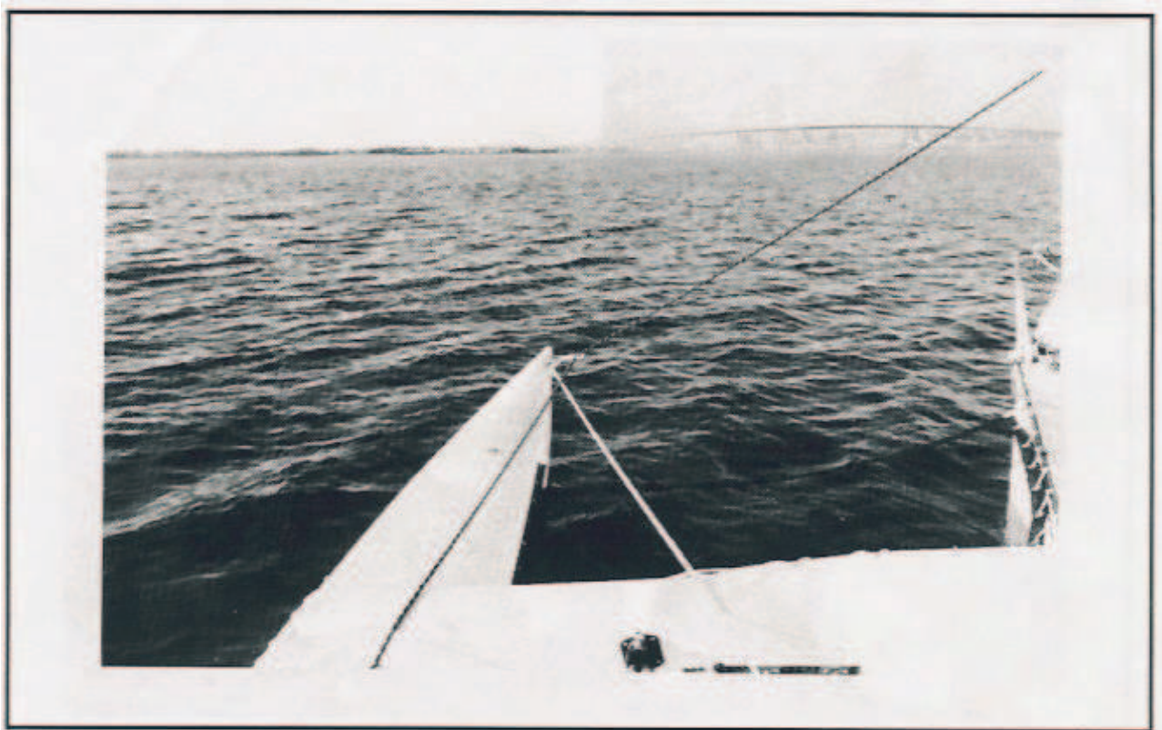
Spinnaker sheet and guy/tweaker line set-up to use the spinnaker poleless. Separate sheets could also be used to the spinnaker clew - one to the bow, and the other to the stern sheeting block.
