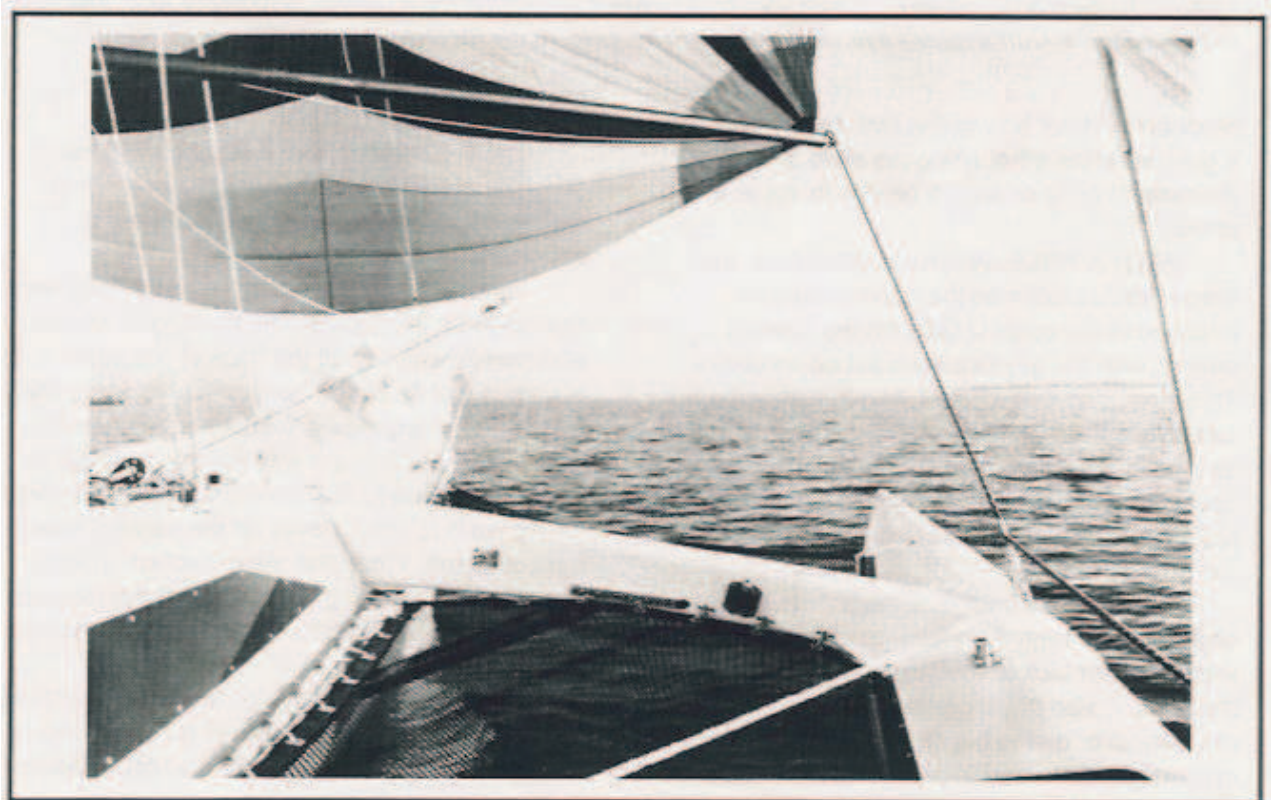
The spinnaker set-up when using the pole. Pole downhaul and topping rift can also be seen.
